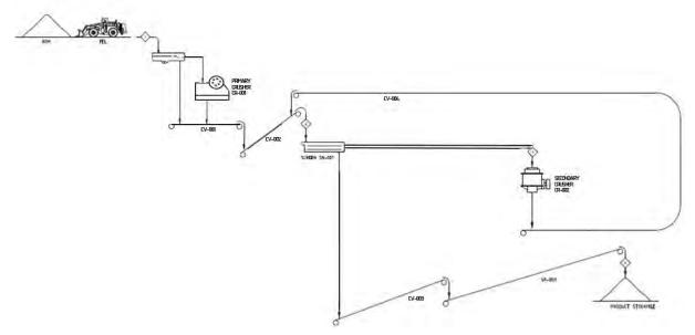
Figure 7 – Process Flow Diagram
