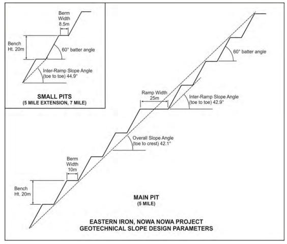
Figure 5 – Geotechnical Slope Design Parameters
